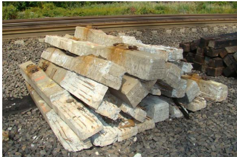
Figure 1: Defective Concrete Ties Removed from Track*
