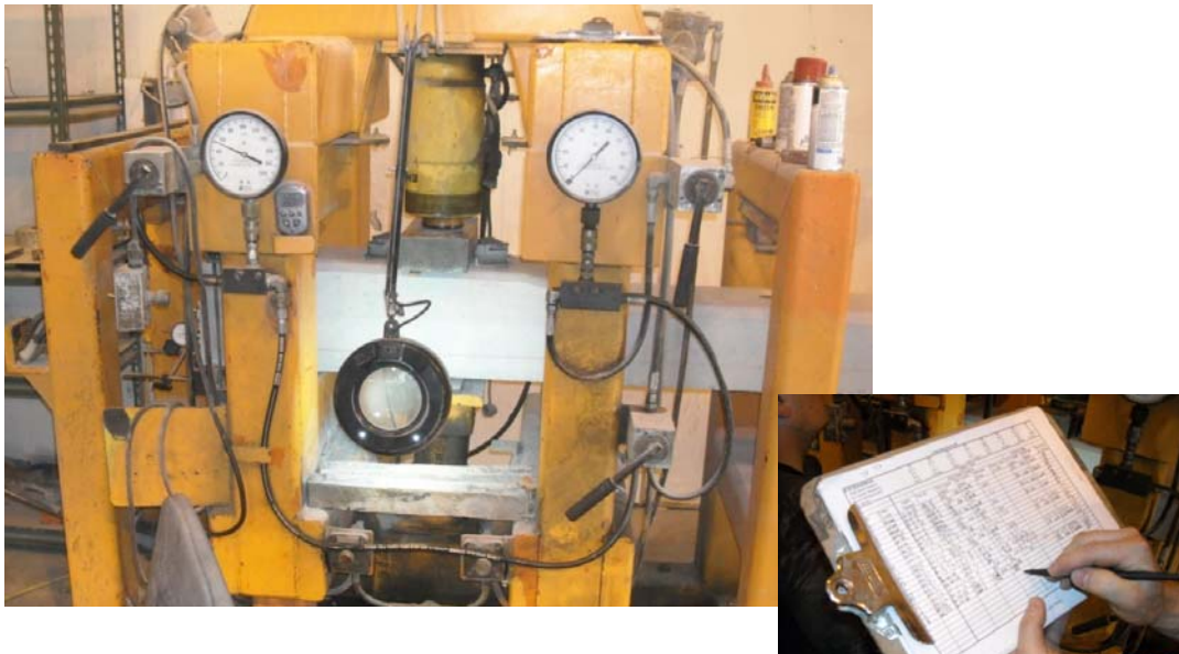
Figure 4: Amtrak Engineer Reviewing Strength Tests of Concrete Ties
